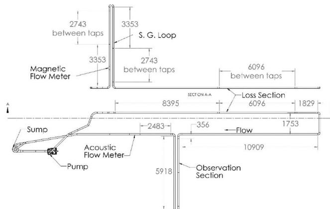
Figure 1. 100 mm Diameter Loop Drawing, units in mm.
