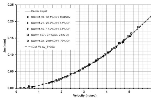
Figure 4. Loss curves ( $j_m$  vs.  $V$ ), expressed in height of *slurry* per length of pipe, measured using the acoustic flow meter, and Four Component model (4CM) predictions at 7% volumetric solids concentration, 35 C, 100 mm loop.
